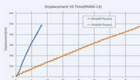
Fig 5. Displacement vs time characteristics during reverse rotation drive (PAM-13)
