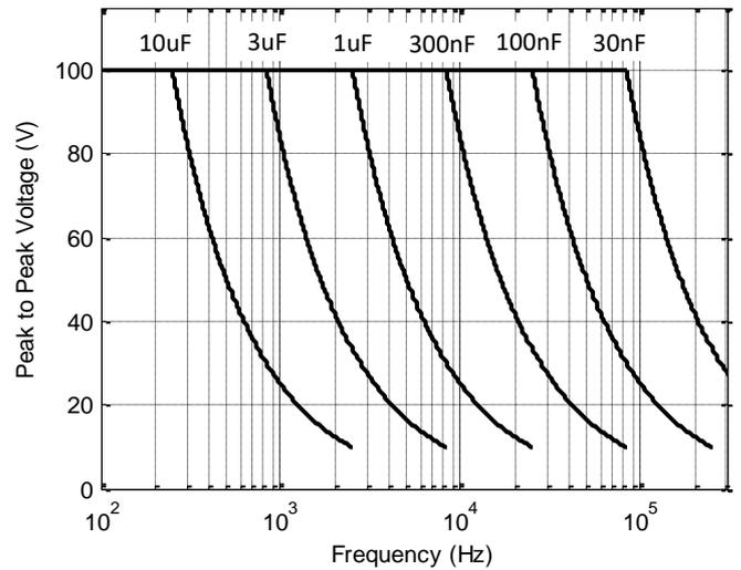
Figure 5. Power Bandwidth (100V Range)
