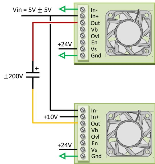
**Figure 9. Bridge configuration achieving  $\pm 200$ V**
