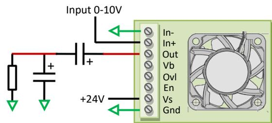
+/-100 V Piezo Driver, see "Bipolar Output Voltage".
