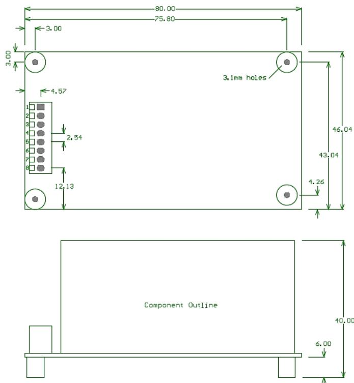
Figure 10. Dimensions (mm)
