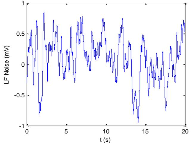
Figure 7. Low frequency output noise (0.03 Hz to 10 Hz)
