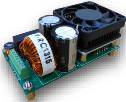
The MX200 is a complete power supply and high-performance linear amplifier module for driving piezoelectric actuators. The MX200 can drive stack actuators; standard piezoelectric actuators; two wire benders; and three-wire piezoelectric benders requiring a bias voltage. Output currents of up to 1 Amp are developed at frequencies up to 100 kHz with less than 100  $\mu\text{V}$  noise (10Hz to 10kHz). Bipolar output voltages up to +/-100V are possible with an external AC coupling capacitor.
